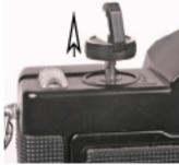
After the film is threaded into the take-up slot, advance the film by releasing the shutter and advancing the knurled knob until the film overlaps on the take up reel. Be sure the film sprocket holes are engaged in the sprockets. Now you can close the camera back. Use the knurled film advance knob to click off a few shots until the number 1 shows in the counter.
